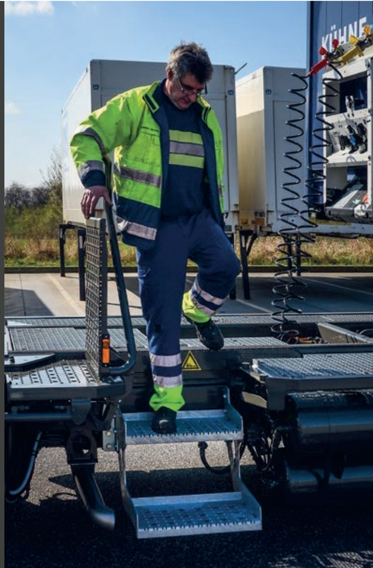
Fold-out stairs on driver's side controlled from the cab for trailer operations.
